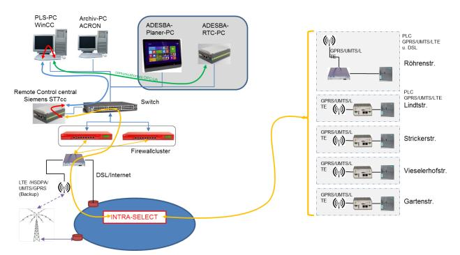
Figure 15 Communication scheme for ADESBA-RTC at the five CSOs (source: SEGNO).
